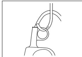
Only after switching off, suspend your heatgun on the hanging ring (5) or stand the tool as in "Hands free use". Leave to
