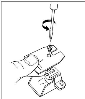
**Note:** Ensure the hole in the scraper is to the left of the screw in the blade holder.
