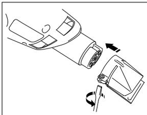
holder engages with the recess on the nozzle. Tighten the blade holder clamp screw.
