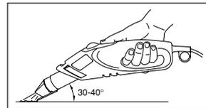
with the surface at an angle of 30-40°.
