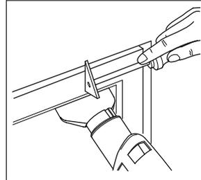
conducted through the metal and can crack the glass. Scrape with the grain of the wood wherever possible. Do not linger on one spot for too long as the surface may char or ignite.
